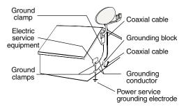
Note: The DIRECTV Receiver must be grounded through the satellite/local antenna cable before plugging into the telephone jack, and it must remain grounded thereafter.
